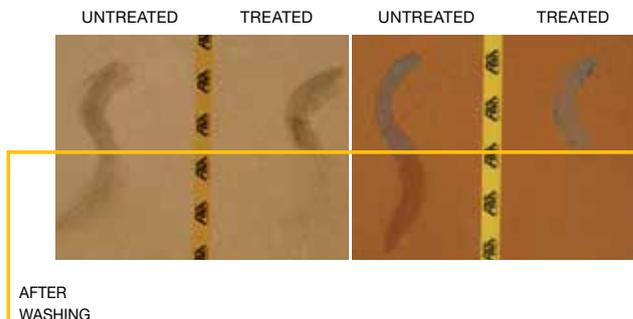
Stain-proofing test carried out on Vicenza stone and terracotta. The untreated section absorbed the grout deep down, which made it difficult to clean after laying. The treated part did not absorb the grout and it was easy to remove with the specific detergent.
